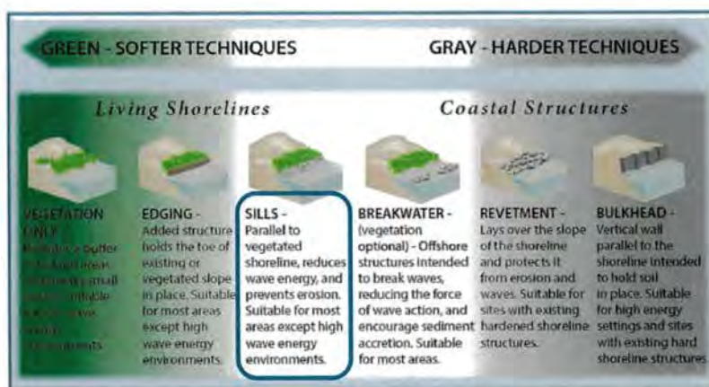
Figure 2 – Green, soft approach to constructing a Living Shoreline from the NOAA 2015 publication, "Guidance for Considering the Use of Living Shorelines."
